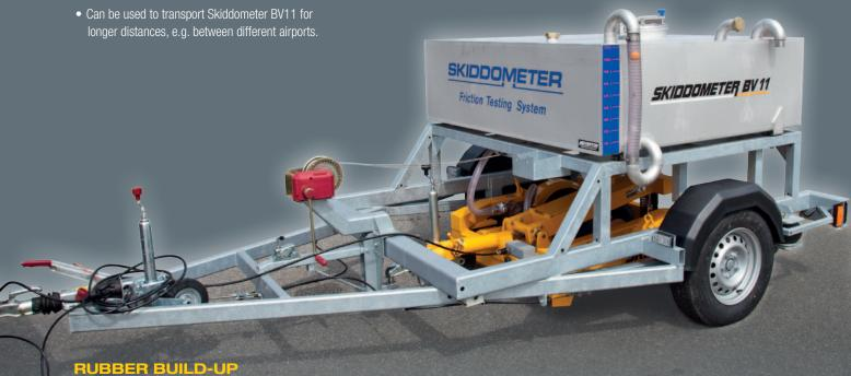
Since wet pavement always yields the lowest friction measurements, Skiddometer should routinely be used on wet pavement, providing the "worst case" measurements for the runway. Removing built up rubber is costly, and requires the runway to be
